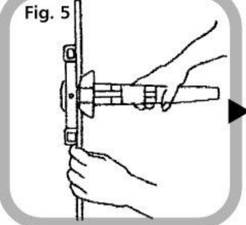
\* Put in the tube with the same direction of the bar, and move the demi-compass to the right angle, then turn down the handle to eject the demi-compass.
