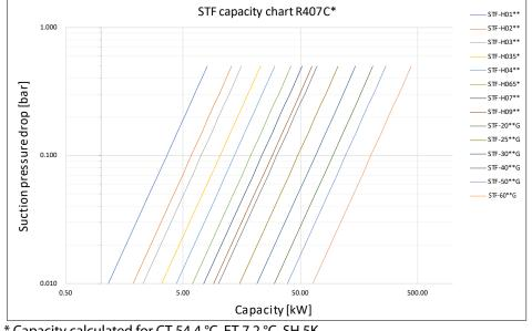
\* Capacity calculated for CT 54.4 °C, ET 7.2 °C, SH 5K
